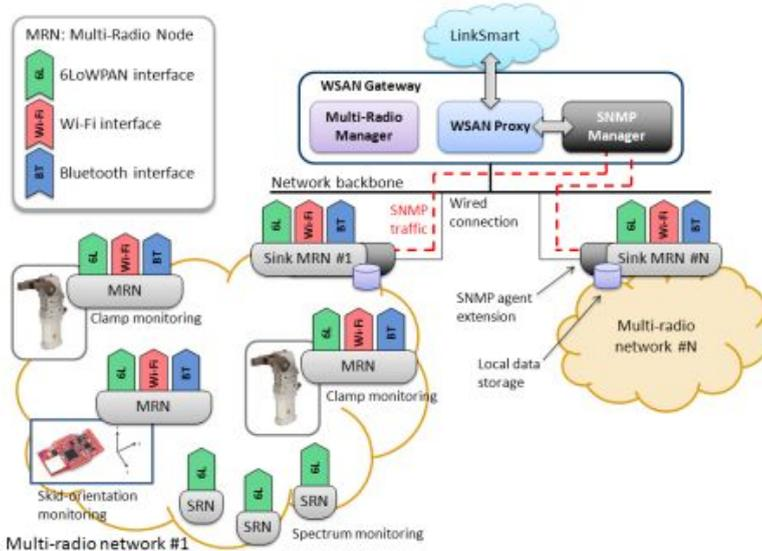
Multi-radio WSAN architecture for manufacturing, integrated into LinkSmart environment.
