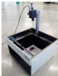
The picture (left) illustrates the setup composed of a wireless smart camera pointing to where a car body is present. The software embedded in the camera is able to identify the position of the car body and send a signal if the position is correct. The software is based in the segmentation of the car body. This segmentation depends on the colour of the object to be inspected, in this case the car body.
