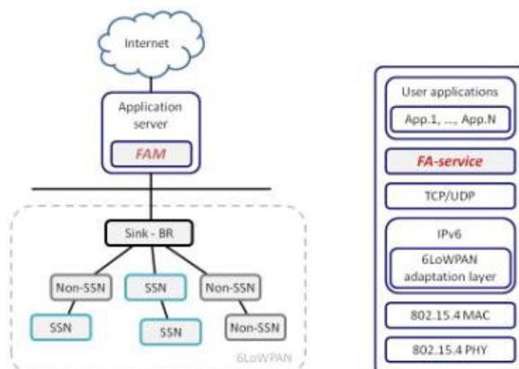
All WSAN data are communicated to the application server for processing, while spectrum sensing information is further processed at a component called the *Frequency Agility Manager* (FAM). The FAM processes the spectrum sensing data and obtains the spectrum occupancy state. If the FAM determines that a critical level of interference is present in the current operating channel (OC), it generates an OC switch command to reallocate the network to the best available channel.
