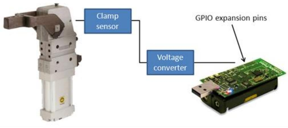
**Figure 12: Interfacing the Telos rev. B sensor node platform with the Tünkers clamp.**
