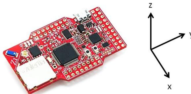
**Figure 11: Layout of the accelerometer axes on the Zolertia Z1 wireless sensor node.**
