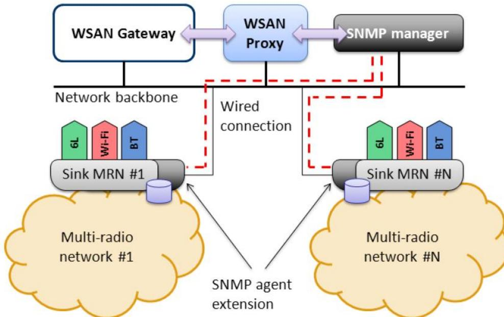
**Figure 9: Final Multi-radio WSA management architecture.**
