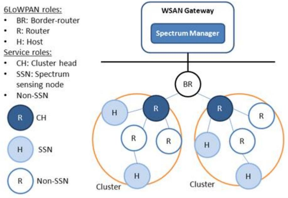
**Figure 7: Single-Radio WSN architecture.**
