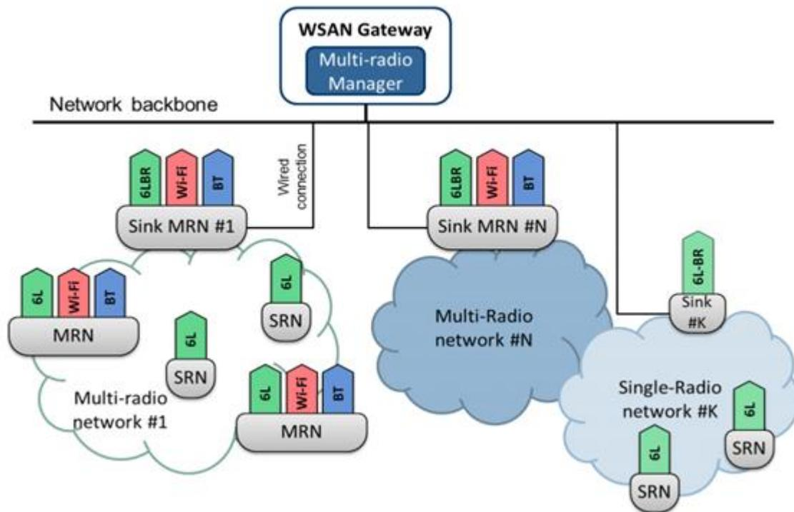
**Figure 8: Multi Radio WSN architecture.**
