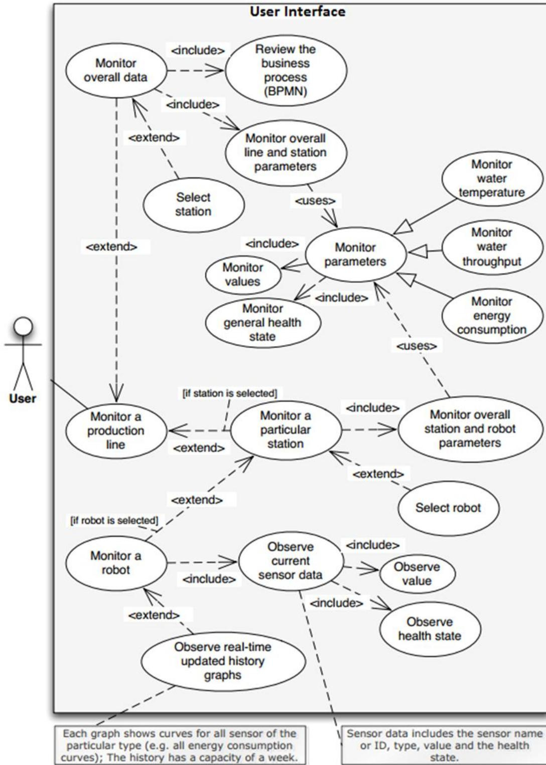
Figure 13: Use case diagram for the user interface.
