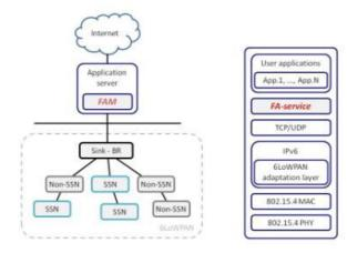
All WSAN data are communicated to the application server for processing, while spectrum sensing information is further processed at a component called the *Frequency Agility Manager* (FAM). The FAM processes the spectrum sensing data and obtains the spectrum occupancy state. If the FAM determines that a critical level of interference is present in the current operating channel (OC), it generates an OC switch command to reallocate the network to the best available channel.
